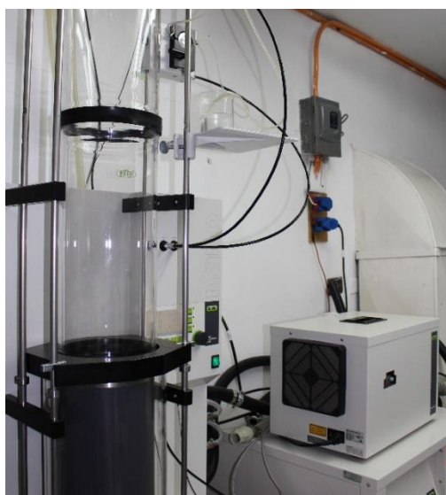
Figura 15 - Nano Spray Dryer, Buchi B-90
