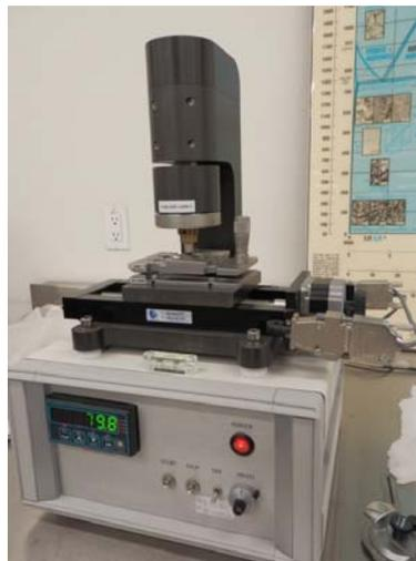
Figura 12. Scratch tester CETR UMT Multi-Specimen Test System.
