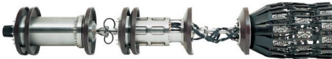
Figura 4. Smartpig, fuente (Reber, Beller, Willems, & Barbian, 2002).
