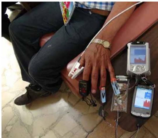
Fig. 8. Oximeters test; Mazimo, Nonin and Oximeter WiFi in a patient.
