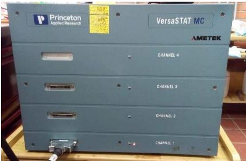
*Figura 21 Potenciostato Versastat 3, Princeton Applied Research*
