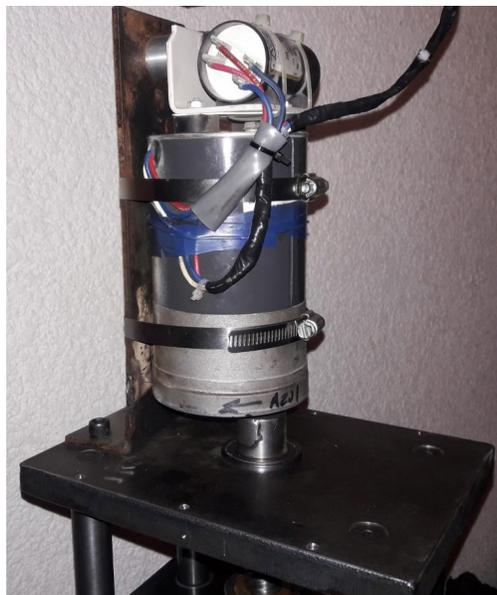
FIGURA 66. MONTAJE MOTORREDUCTOR
