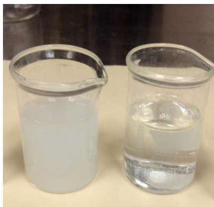
Figure 48. Sedimentation test for the treated TiO 2 . Untreated TiO 2 in water, left, and treated TiO 2 in water, right.
