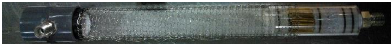
Figure 29. Photograph of the external electrode of the reactor, a stainless-steel wired mesh.
