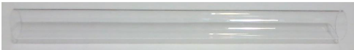
Figure 28. Photograph of the cylindrical Quartz crystal glass used as the dielectric surface of the reactor.
