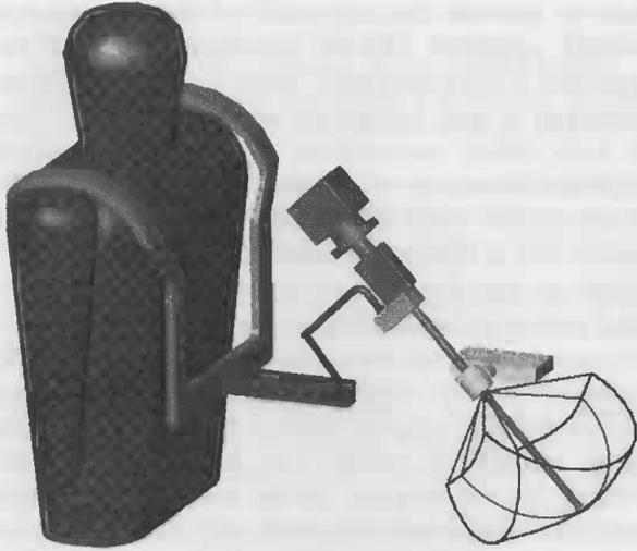
FIGURE 4. Virtual work space of the mechatronic system using Visual Nastram 4D™ and Mechanical Desktop™. The point of entry is invariant throughout the entire virtual navigation.
