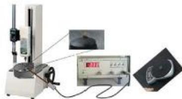
Fig. 5. Magnetic levitation experimental set.
