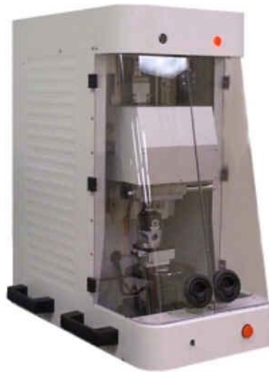
Figura 23. Scratch tester CETR UMT Multi-Specimen Test System.
