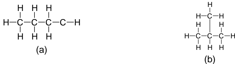
Figura II.15. El butano ( C_4H_{10} ) puede ser: (a) butano normal ( n-C_4H_{10} ) o (b) isobutano ( i-C_4H_{10} ). [45]
