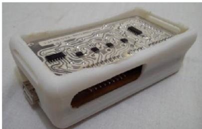
Fig. 4 – The integration of the device in a 3D printed protection box made of polylactic acid without the lid to show the PCBs.
