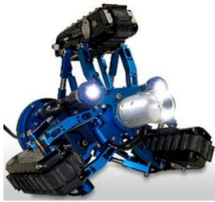
Figura 2. Pipeline inspection underwater ROV. VT100 Vertical Crawler. INUKTUN.
