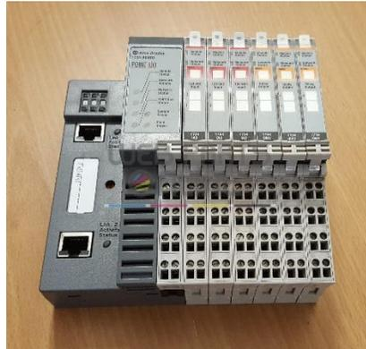
Figura 3.11: Modulo Point I/O.
