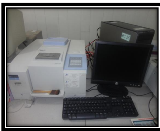
Figura 7. FTIR Perkin Elmer Spectrum 100
