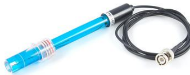
Figura 3. 24 Sensor de pH asp200-1 m-bnc
