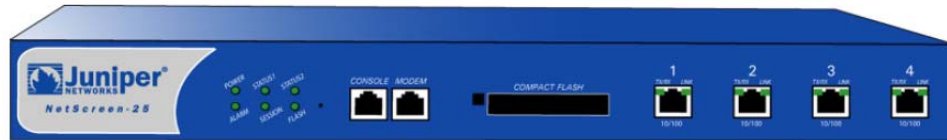
Figura 3.18 Vista frontal del Firewall Netscreen-25
