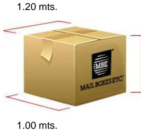
$$PV = \frac{L \times A \times H}{6000 \text{ cm}^3 / \text{kg}}$$
