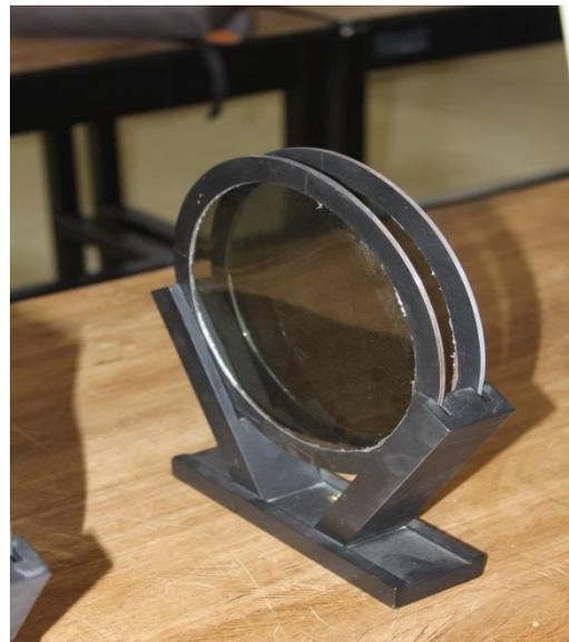
Fig.3.9 Polariscopio Circular.
