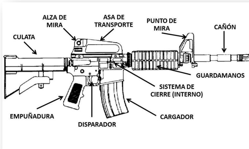
**Figura I.2.-** Fusil (carabina) M4 A1 calibre 5.56 x 45 mm [M4A1 Technical manual, 1997].
