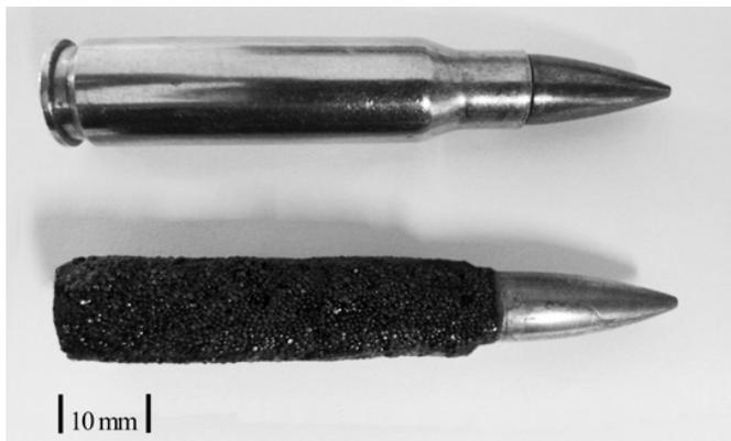
Figure 3. Ammunitions 7.62 x 51 mm FMJ and 7.62 mm caseless-coreless prototype.
