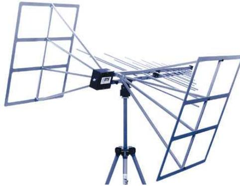
Fig. 1.9 Antena Híbrida (BiConiLog).
