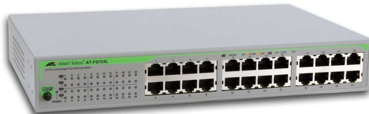
Figura 3.30. Switch perimetral no gestionable
