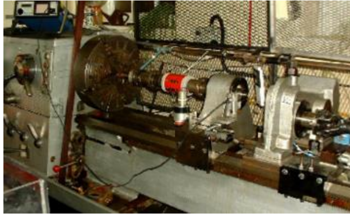
Figura 2.12 Maquina de discos encontrados SUROS (Sheffield University Rolling Sliding)
