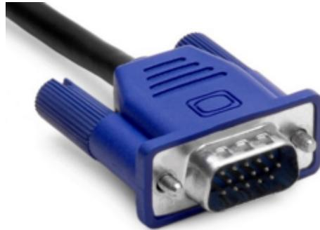
Figura 26. Conector VGA (Video Graphic Array).
