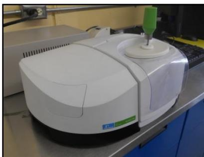
**Figura 6. Espectroscopio FT-IR Spectrum Two (UATR TWO).**
