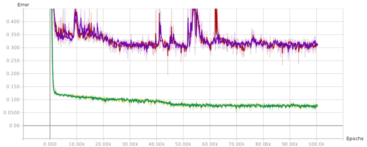
Figure 5.3: Both models copy task learning error plot for a 10 \times 5 size sequence. ■ Neural Turing Machine test. ■ Neural Turing Machine train. ■ Differentiable Neural Computer test. ■ Differentiable Neural Computer train.
