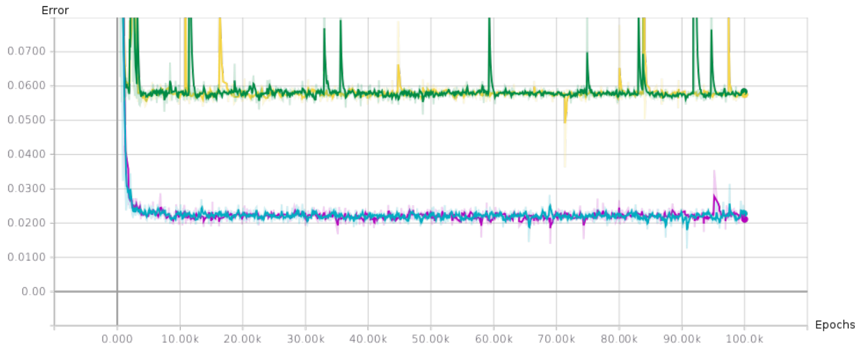
Figure 5.6: Both models associative recall task learning error plot for a 10 \times 10 size sequence. ■ Neural Turing Machine test. ■ Neural Turing Machine train. ■ Differentiable Neural Computer test. ■ Differentiable Neural Computer train.
