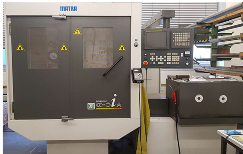
Fig. 3.2. Fanuc Robocut \alpha -0iA EDM machine.
