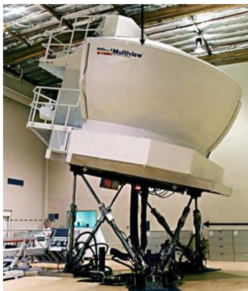
Figura 12 - Advanced Concept Flight Simulator (ACFS) desarrollado por CVSRF [16].
