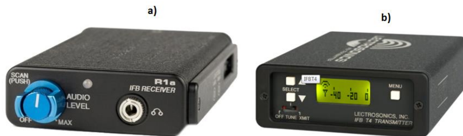
Figura 3.38. a) Receptor R1a, b) Transmisor IFB T4
