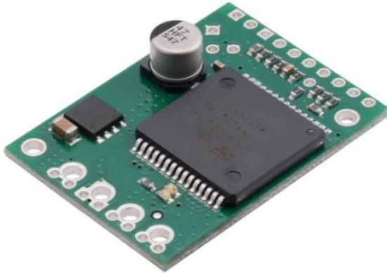
This carrier board for ST's VNH5019 motor driver IC operates from 5.5 to 24 V and can deliver a continuous 12 A (30 A peak). It works with 2.5 to 5 V logic levels, supports ultrasonic (up to 20 kHz) PWM, and features current sense feedback (an analog voltage proportional to the motor current). Along with built-in protection against reverse-voltage, over-voltage, under-voltage, over-temperature, and over-current, these features make this product a great general-purpose motor driver.
