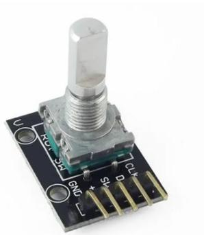
The Keyes KY-040 rotary encoder is a rotary input device (as in knob) that provides an indication of how much the knob has been rotated AND what direction it is rotating in. It's a great device for stepper and servo motor control. You could also use it to control devices like digital potentiometers. Pulses per rotation are 20, and consumption current are 10mA.
