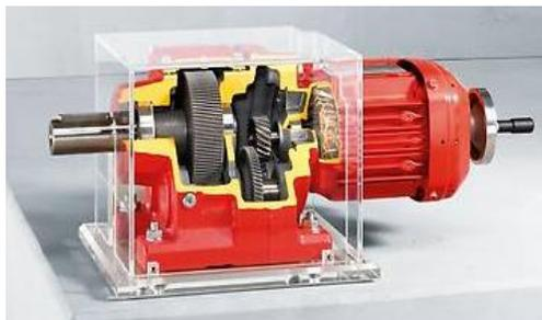
Figura 9. Motorreductor [21].
