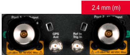
For N9950/51/52/60/61/62B, N9953/63B (54 GHz) are with 1.85 mm (m) connectors.
