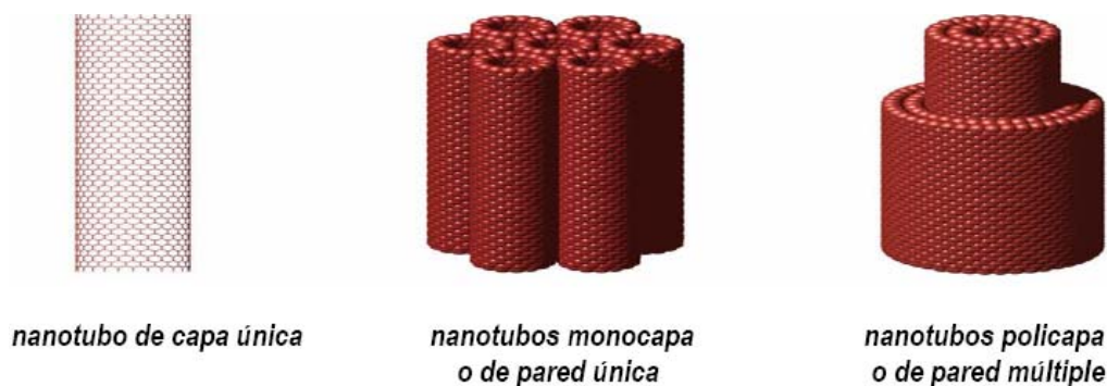
Figura 3.12:-Formas enrolladas de nanotubos de carbono de pared única o múltiple. (Fuente: Q. Wang y J. K. Jonson, 1999 “Molecular simulation in single-walled carbon nanotubes and idealized carbon slip pore”)
