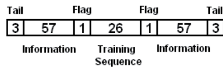
Figura 2.8 Trama de Canal de Trafico (Traffic Channel CH)
