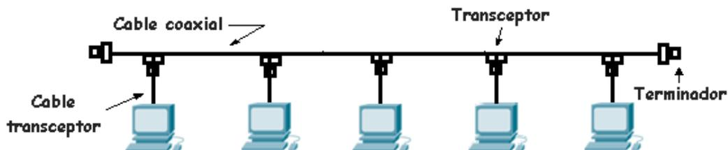
Figura 1.5.- Ethernet Thick Ethernet.
